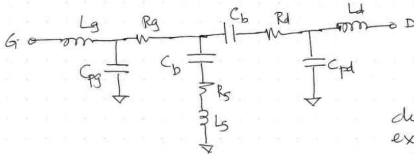
$C_b \rightarrow$  fringing capacitance due to depletion layer extension at each side of gate.
