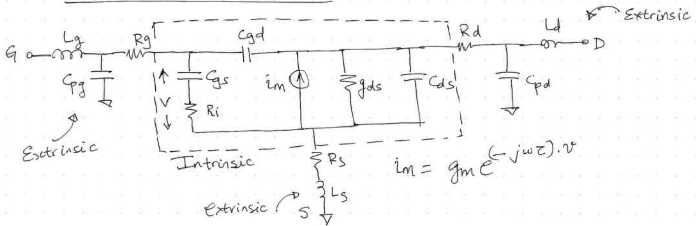
The Y-parameters of the intrinsic device are:
