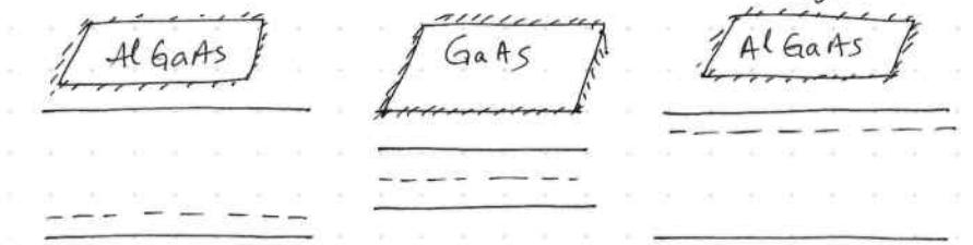
Thickness of sandwiched GaAs layer is in our control
