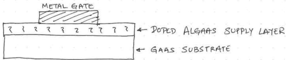
Instead of doping the channel directly, the adjacent AlGaAs layer is doped. The wide bandgap of the doped supply layer ensures that the mobile electrons populate the GaAs channel. At least for low fields, the mobile electrons suffer less scattering because conduction occurs in an undoped medium. The HEMT has been superseded by the pseudomorphic HEMT (pHEMT) but was an important stepping stone in its development.
