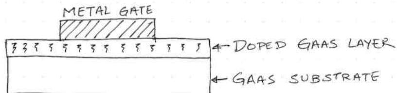
A doped GaAs layer has a lower band gap energy, and when contacted with an ~~an~~ undoped GaAs substrate (with higher band gap energy), the electrons from the GaAs substrate move into the doped GaAs layer and makes it a conducting channel.
